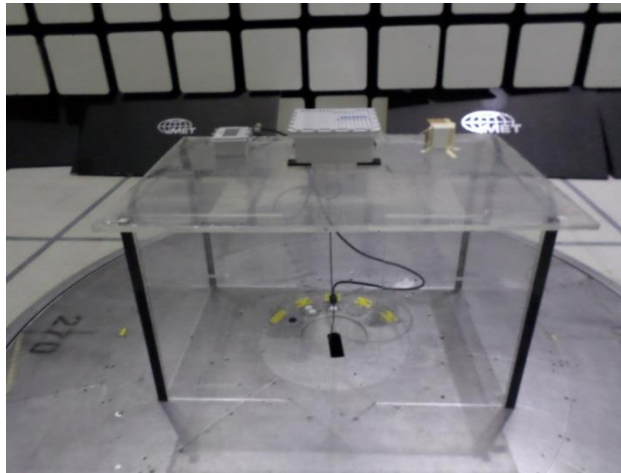
Photograph 1. Radiated setup, 30M-1GHz front view
