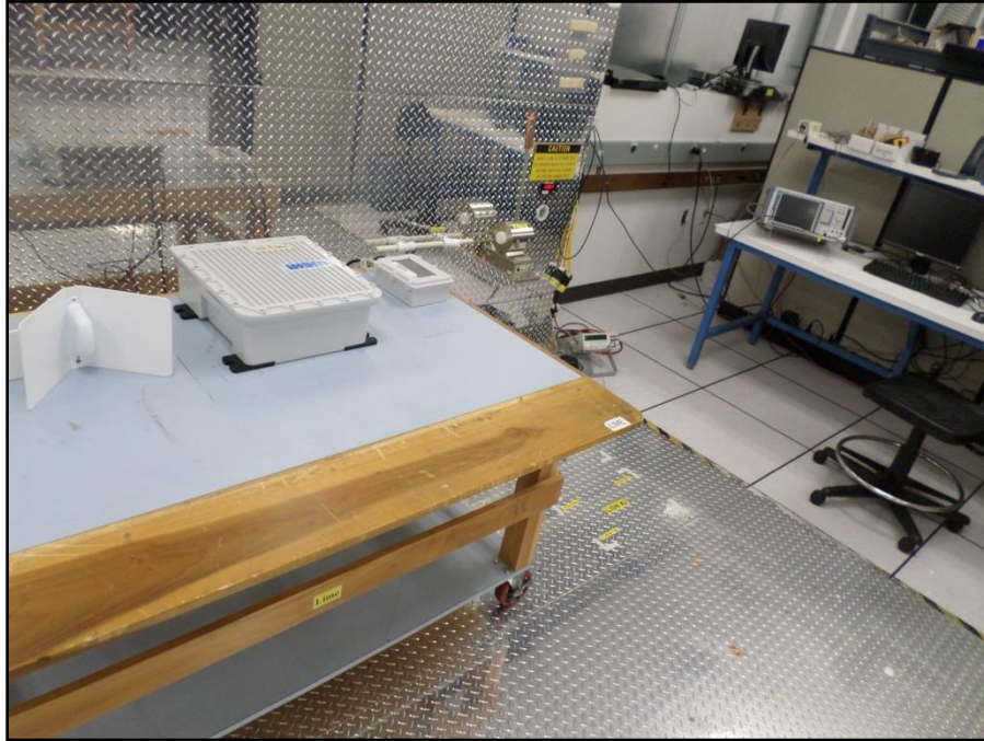
Photograph 10. Conducted Emissions, 15.207(a), CEV Station Setup
