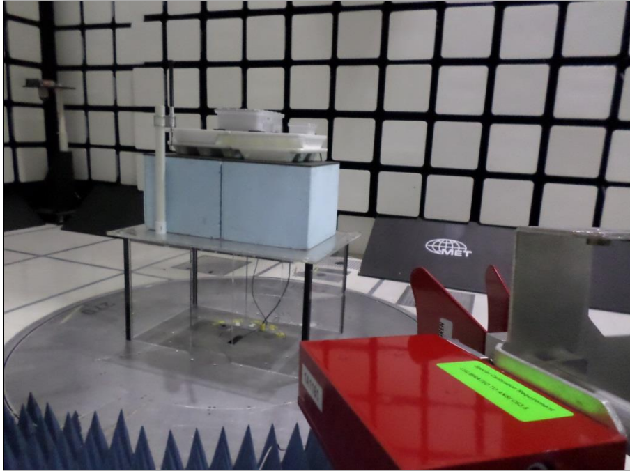
Photograph 11. Radiated Spurious Emissions, 6dBi, 18 - 40 GHz, Test Setup, Antenna
