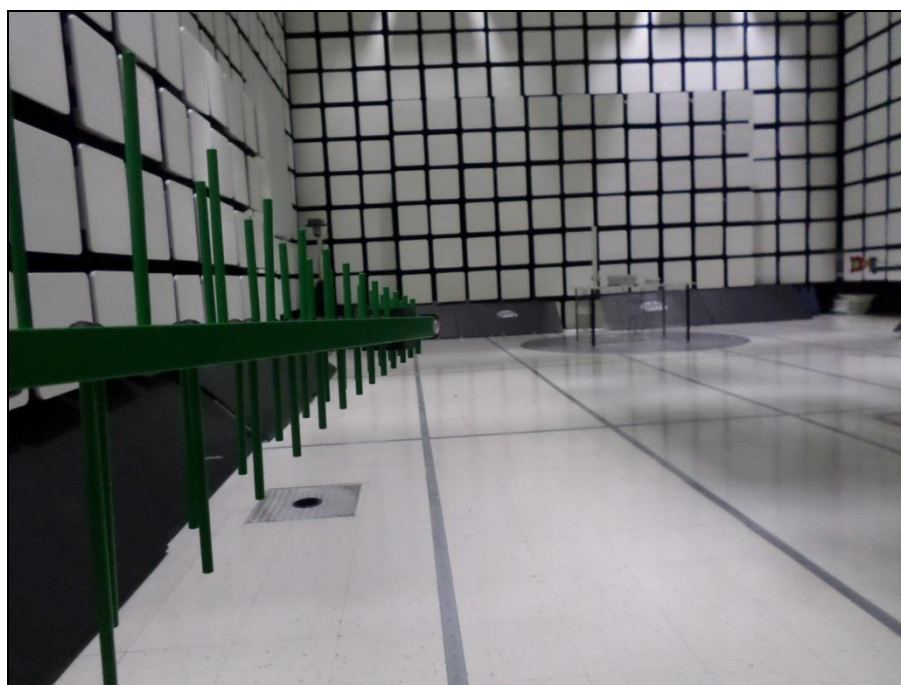
Photograph 8. Radiated Spurious Emissions, 6dBi, 30 MHz - 1 GHz, Test Setup, Antenna
