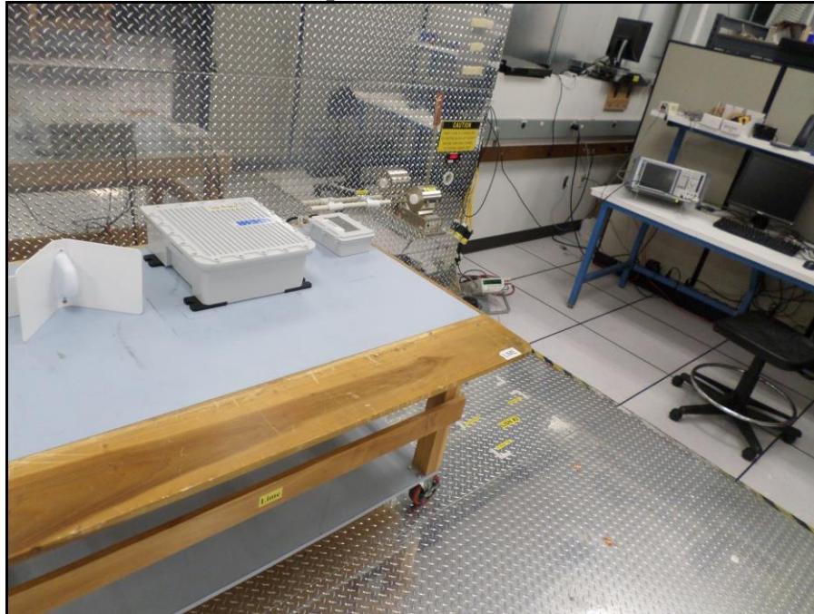
Photograph 1. Conducted Emissions, 15.207(a), CEV Station Setup
