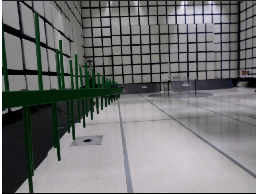
Photograph 9. Radiated Spurious Emissions, 6dBi, 30 MHz - 1 GHz, Test Setup, Antenna
