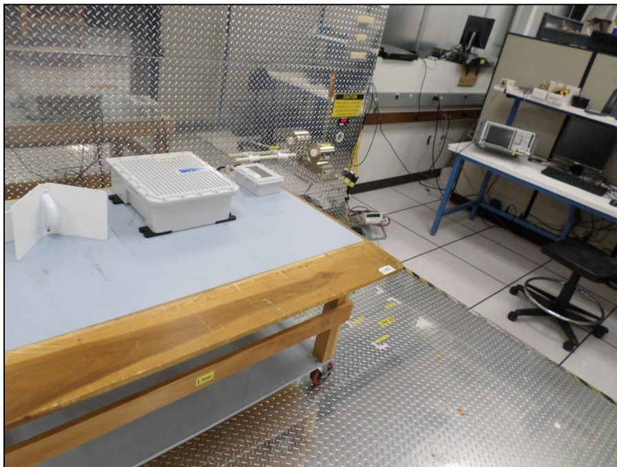
Photograph 1. Conducted Emissions, 15.207(a), CEV Station Setup
