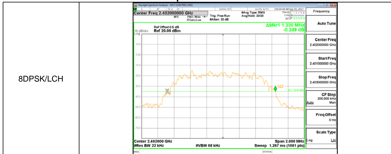
Test Graph: 20dB bandwidth
