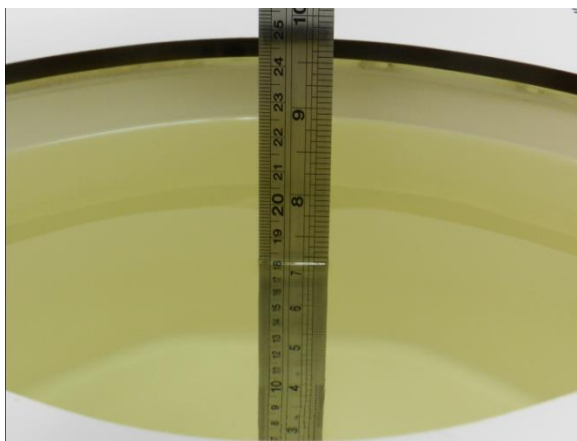
Fig 10.1 Photo of Liquid Height for Body SAR
