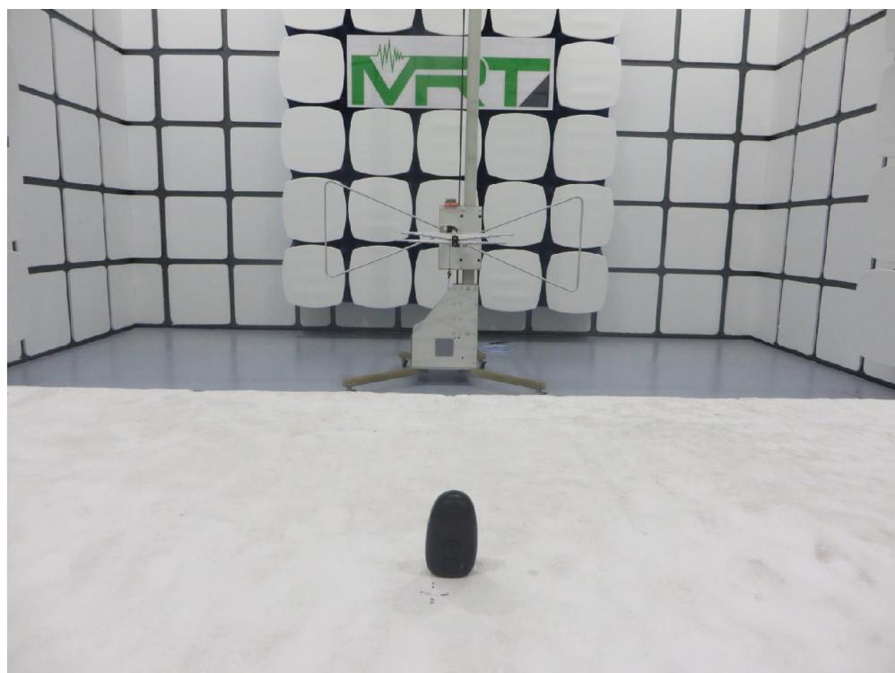
Description: Radiated Emission Test Setup for 1G ~ 18GHz
