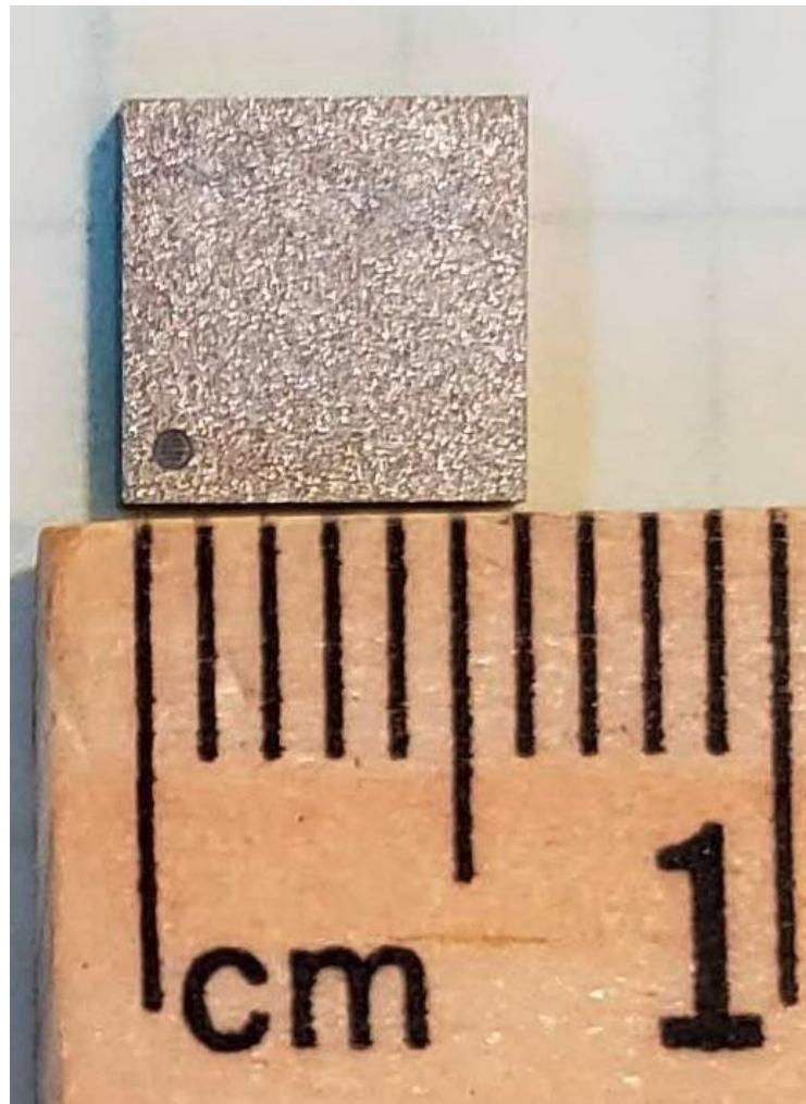
Due to its size of 0.6 cm \* 0.6 cm there is not enough space to place the required certification identification in a readable size (min 4 point) on the device itself.
