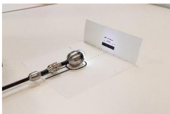
Fig. 49: Calibration with calibration template
