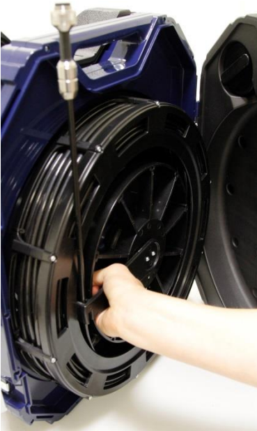
Fig. 74: Grasping the end of the rod and the viper
