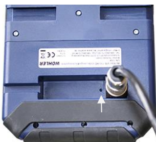
Fig. 69: Reset hole indicated by an arrow
