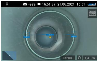
Fig. 46: Warning triangle under distance indicator
