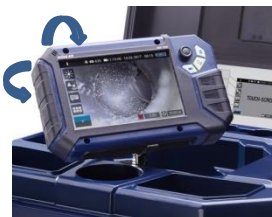
Fig. 12: You can turn and tilt the monitor
