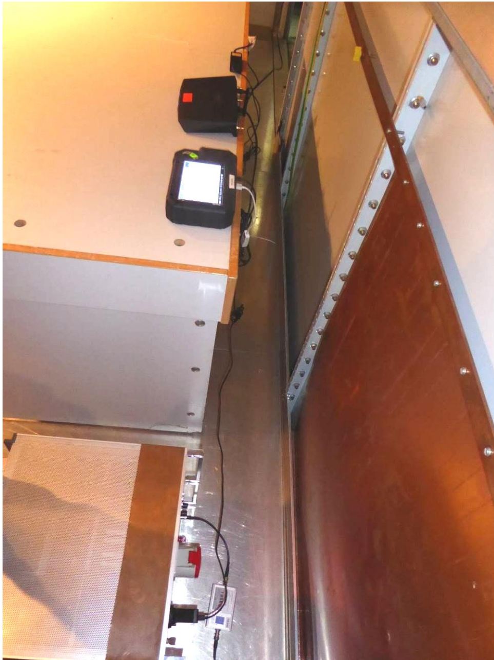
180488_radio_08: Test setup – conducted emissions on power supply lines
