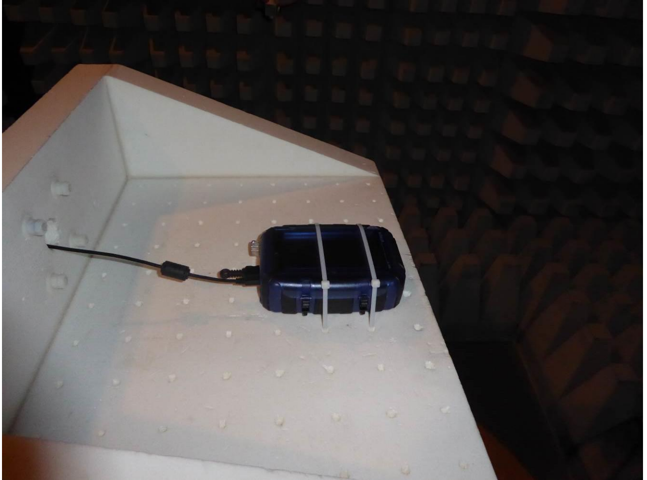
170475_02.JPG: Test setup – radiated test in anechoic chamber
