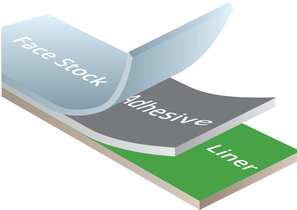
**Face Stock:** 2.4 mil topcoated gloss green polyimide film offering excellent chemical resistance combined with superior high heat resistance. The material will not curl and is designed to survive high temperatures of lead-free solder processes.
