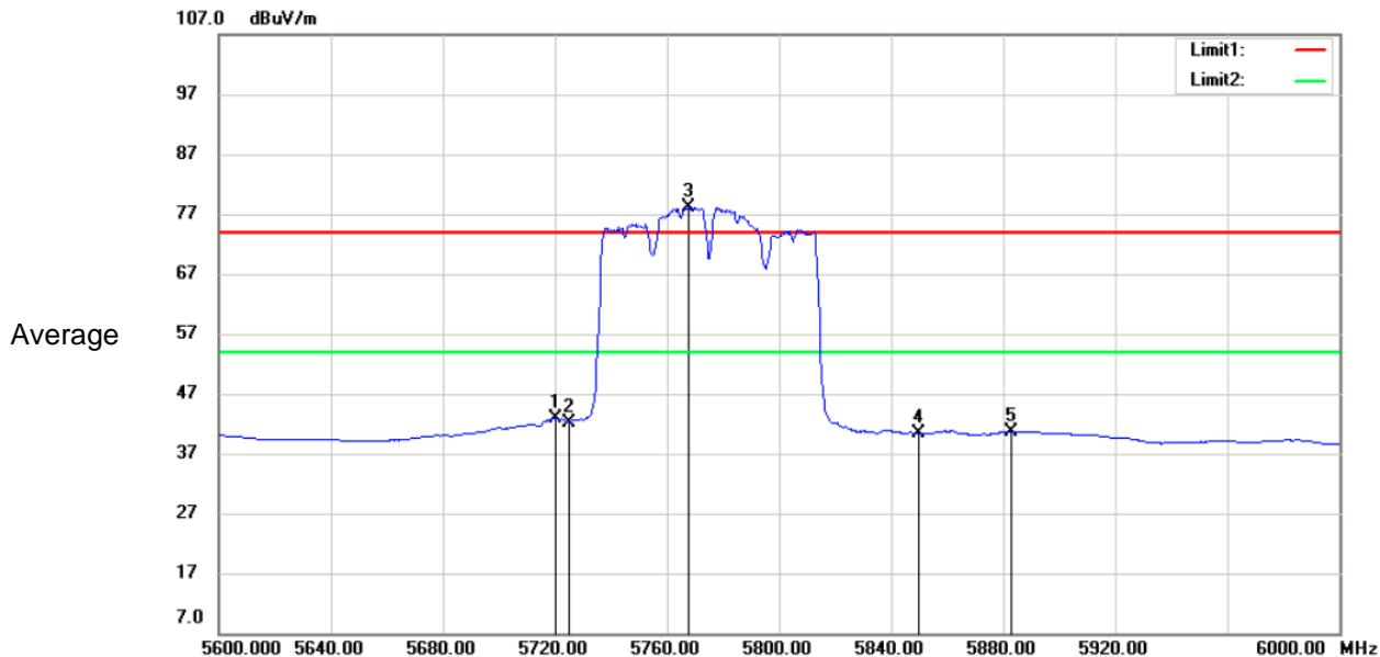
Remark: 1. Test Level = Receiver Reading + Antenna Factor + Cable Loss- Preamplifier Factor
