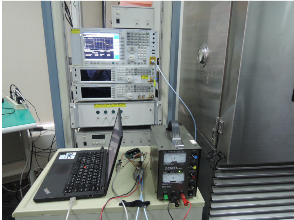
Photograph 5: Set-up for Conducted testing
