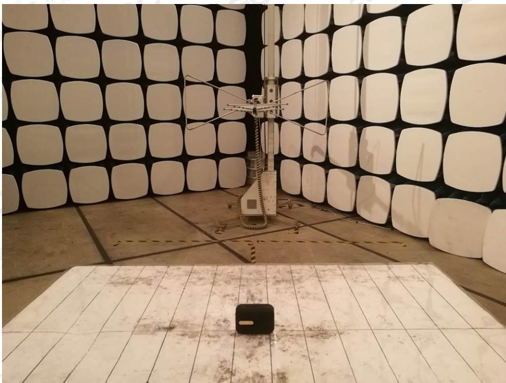
FCC RADIATED EMISSION TEST SETUP
