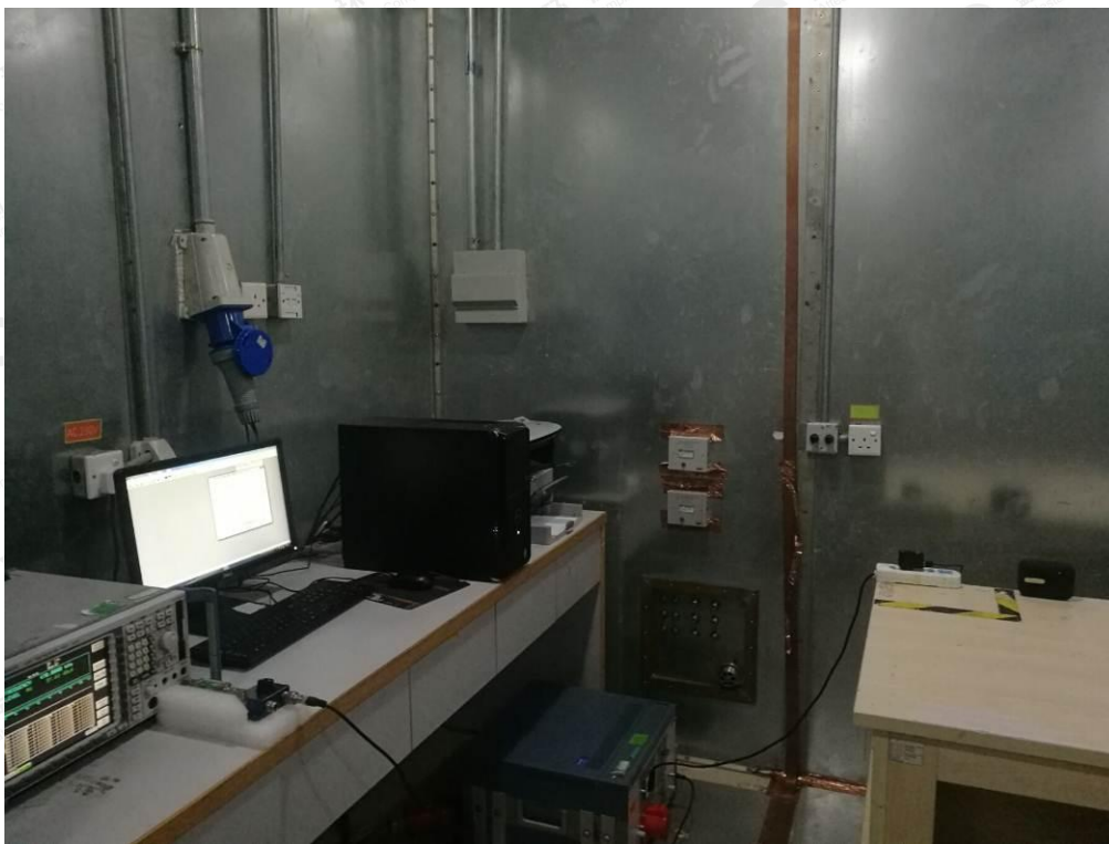
FCC RADIATED EMISSION TEST SETUP
