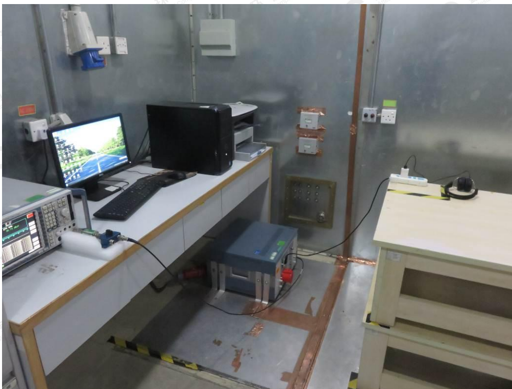
FCC RADIATED EMISSION TEST SETUP
