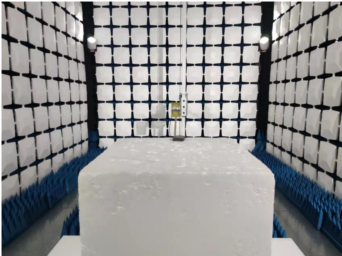
Above 1GHz for radiated emission test setup
