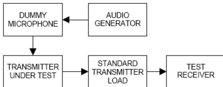
Test at five different modulating frequencies (100Hz, 300Hz, 500Hz, 1KHz, 2.5kHz, 5kHz, 10kHz, 15kHz), the output level of the audio generator was varied up to 1V and the FM deviation level was recorded.
