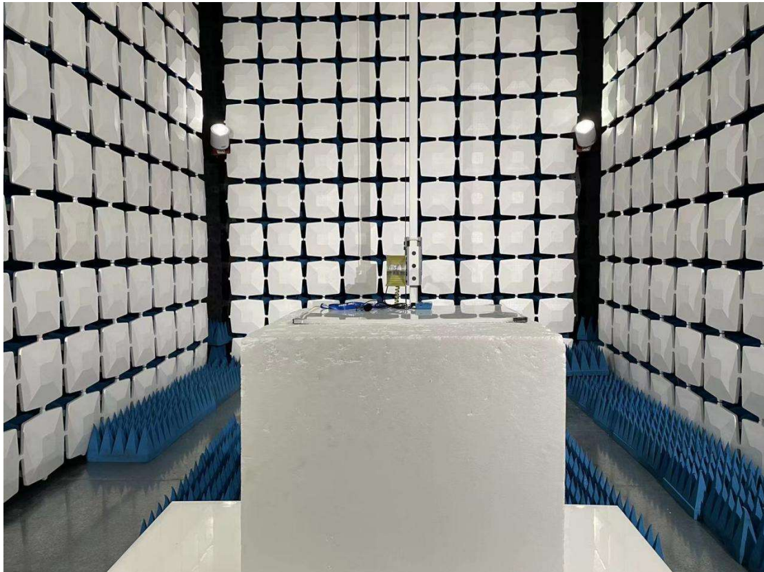
Above 1GHz for radiated emission test setup
