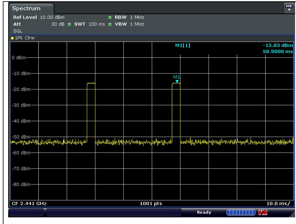
In AFH mode, the minimum hopping frequencies are 20, to get the longest dwell time 3DH5 packet is observed;
