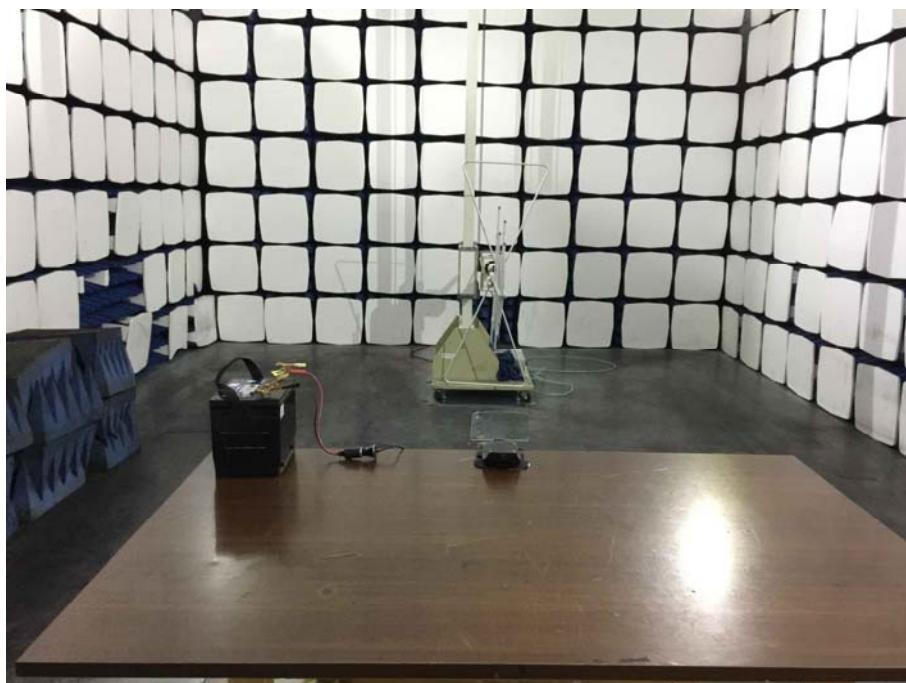
**Radiation Emission Test Setup (Above 1GHz)**
