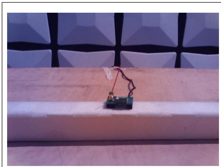
**Radiated Spurious Emission: Half Wave Wire Antenna, <1 GHz**
