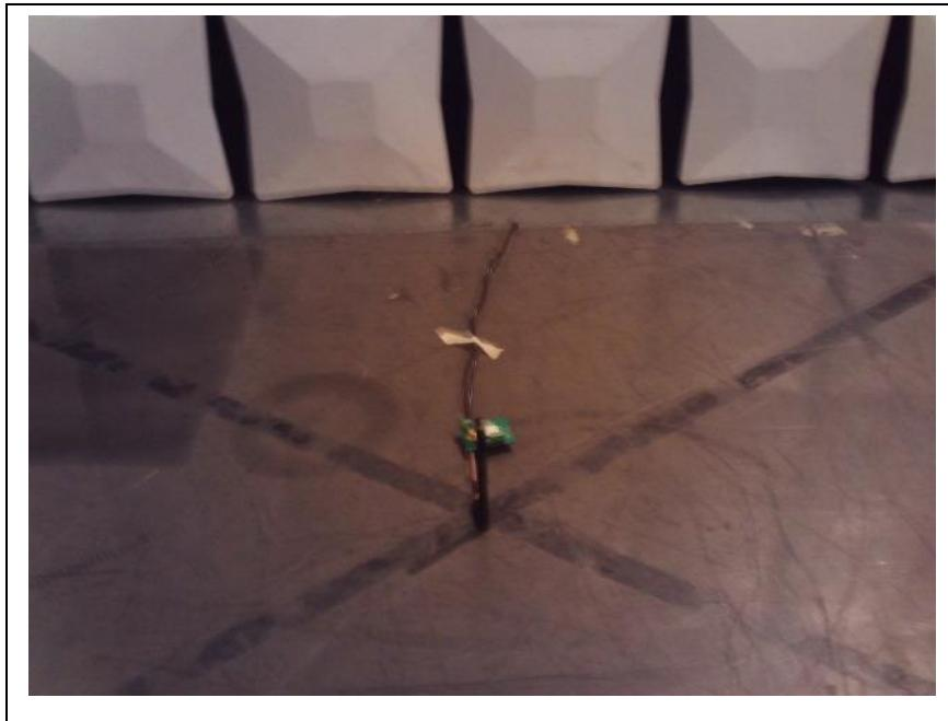
**Radiated Spurious Emission: Half Wave Wire Antenna, >1 GHz**
