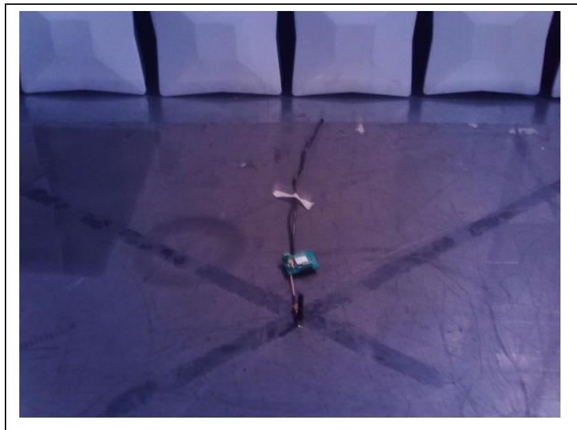
**Radiated Spurious Emission: Quarter Wave Wire Antenna, >1 GHz**
