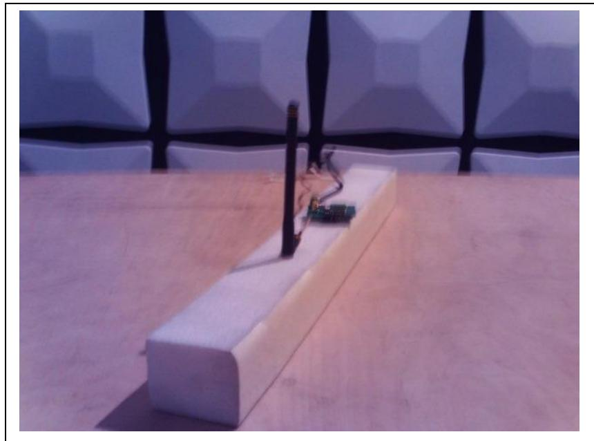
**Radiated Spurious Emission: Quarter Wave Wire Antenna, <1 GHz**
