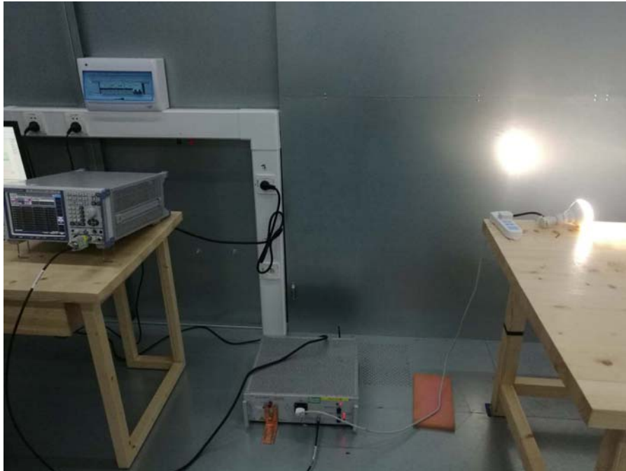
Radiated emission test setup
