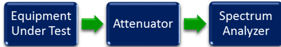
Figure 3. Occupied Bandwidth Test Setup
