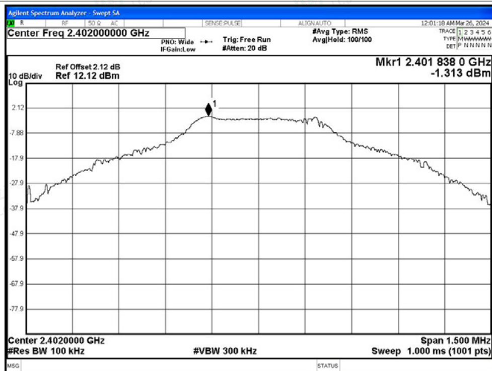
Tx. Spurious NVNT 1-DH5 2402MHz Ant1 Emission
