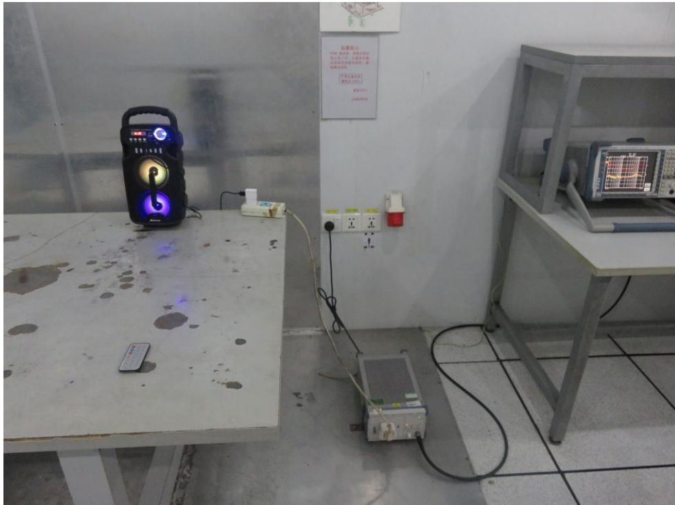
Photo of Conducted Emission Measurement
