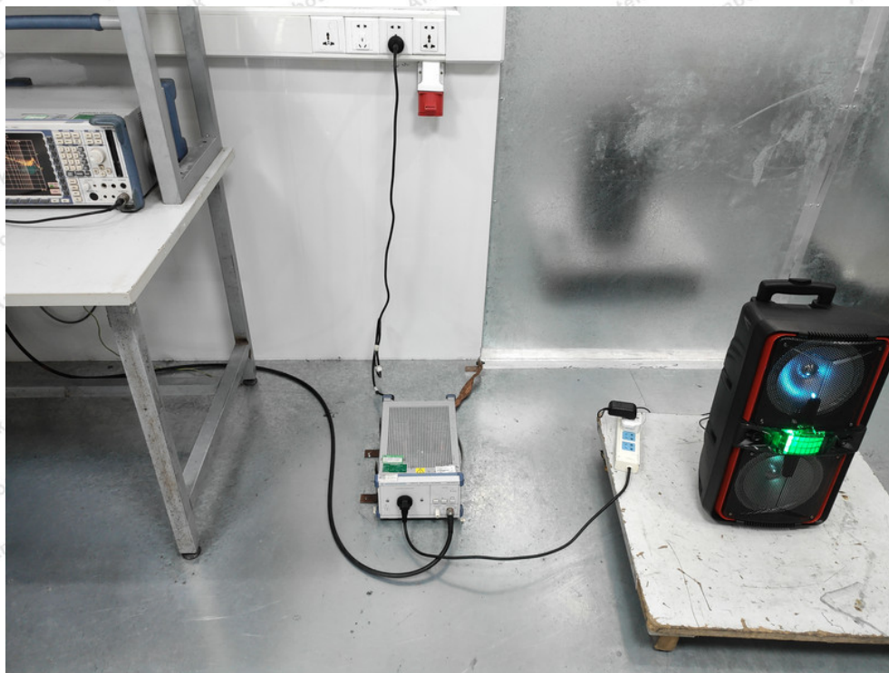
Photo of Conducted Emission Measurement
