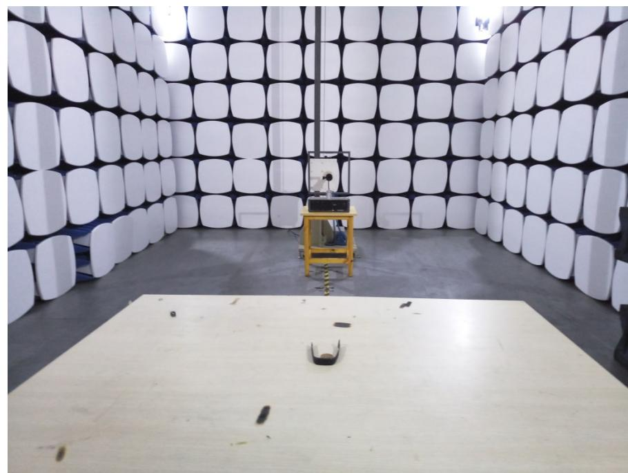
**Radiation Emission Test Setup (30MHz to 1GHz)**
