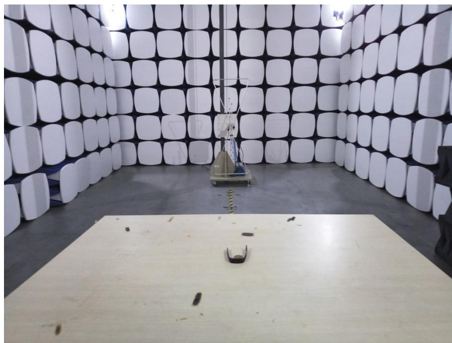
**Radiation Emission Test Setup (1GHz to 18GHz)**
