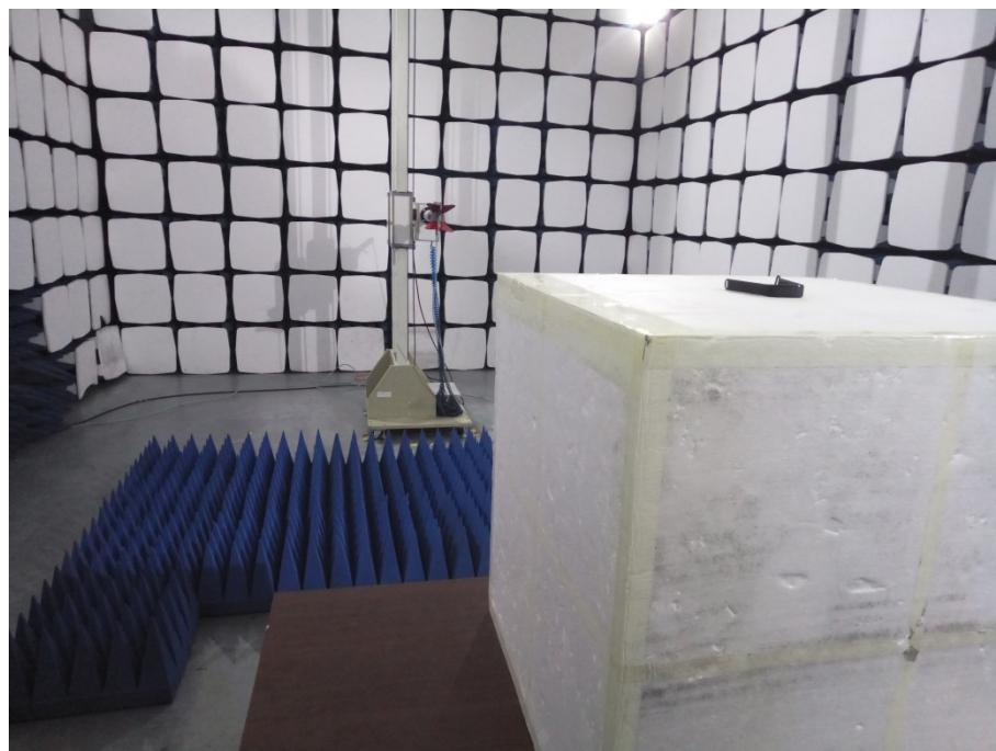
**Radiation Emission Test Setup (Above 18GHz)**
