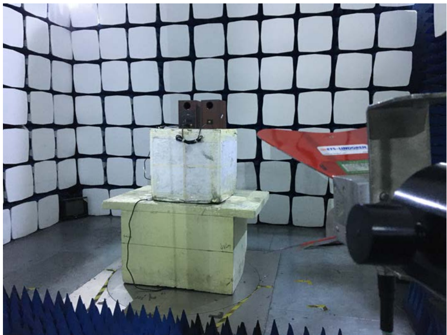
Radiation Emission Test Setup (1GHz to 18GHz)
