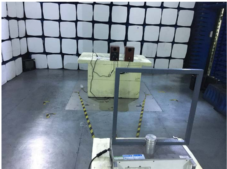
Radiation Emission Test Setup (Below 30MHz)
