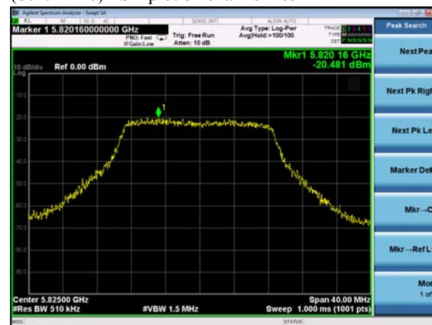
(802.11n20) PSD plot on channel 165
