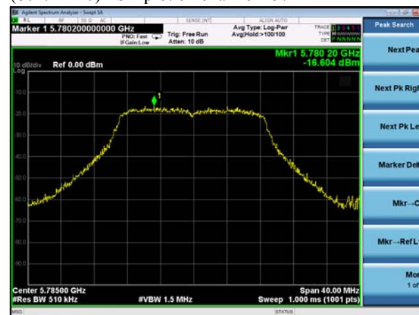
(802.11n20) PSD plot on channel 157
