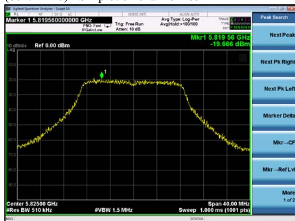
(802.11n20) PSD plot on channel 165
