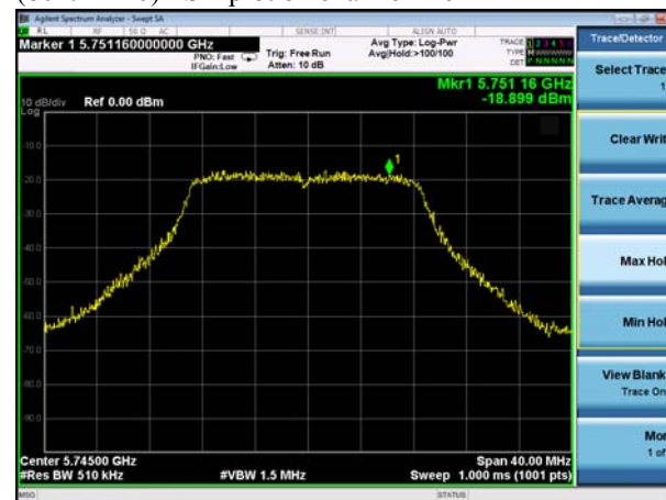
(802.11n20) PSD plot on channel 149
