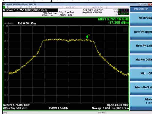
(802.11n20) PSD plot on channel 149
