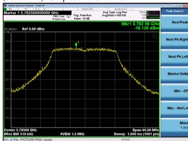
(802.11n20) PSD plot on channel 157
