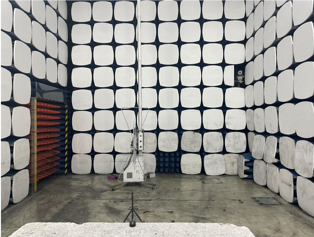
FCC Radiated Emission Test Setup-above 1GHz
