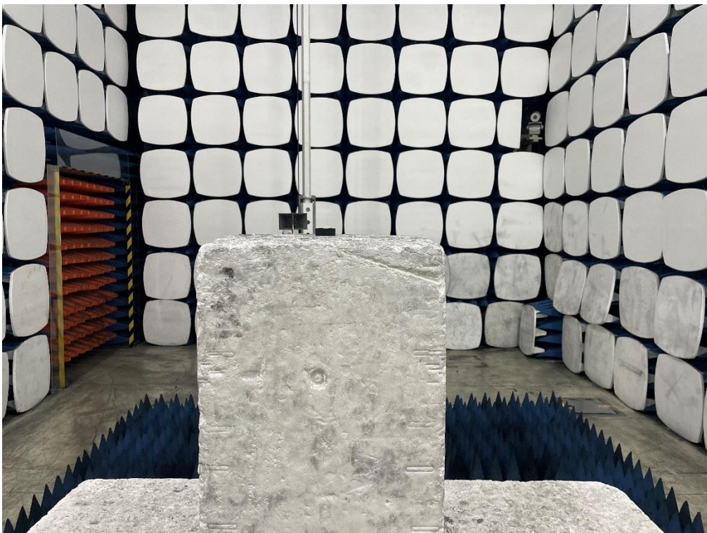
FCC Radiated Emission Test Setup-above 1GHz
