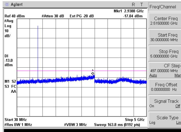
Conducted Emission Transmitting Mode CH 128
