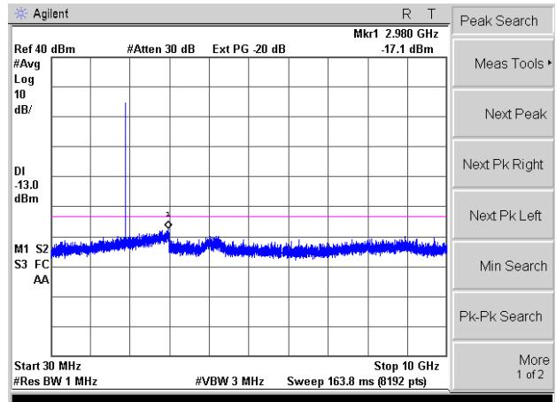
Conducted Emission Transmitting Mode CH 661
