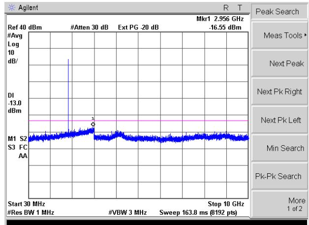
Conducted Emission Transmitting Mode CH 251
