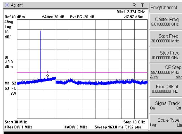
Conducted Emission Transmitting Mode CH 251
