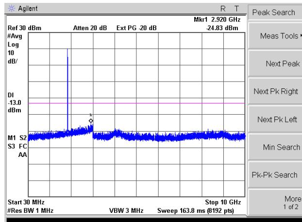
Conducted Emission Transmitting Mode CH 4233
