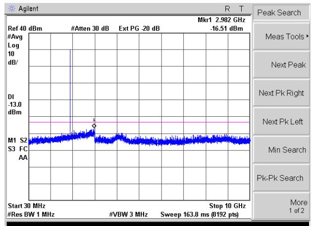
Conducted Emission Transmitting Mode CH 661
