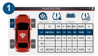
After selecting Verify IDs/DTC Codes, trigger each sensor of the vehicle. In this example the RR sensor is not triggering.
