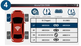
Continuing on to Verify IDs, this example shows that there is an ID stored in the vehicle but triggering the sensor shows no sensor detected. The sensor needs to be replaced.
