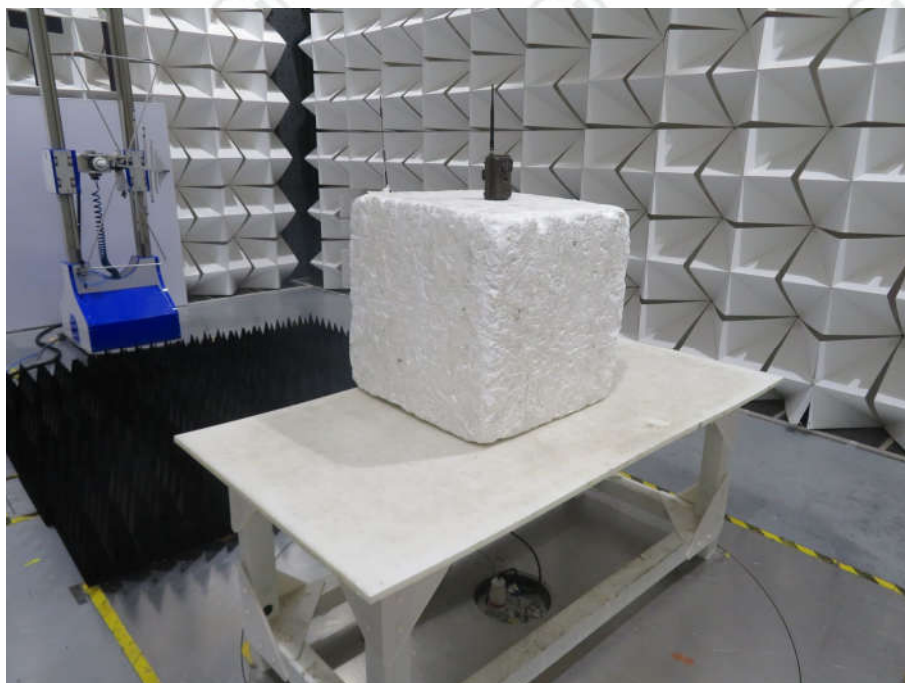
Radiated spurious emission Test Setup-1(Below 1GHz)
