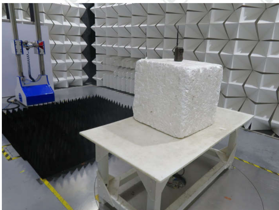
Radiated spurious emission Test Setup-2(Above 1GHz)
