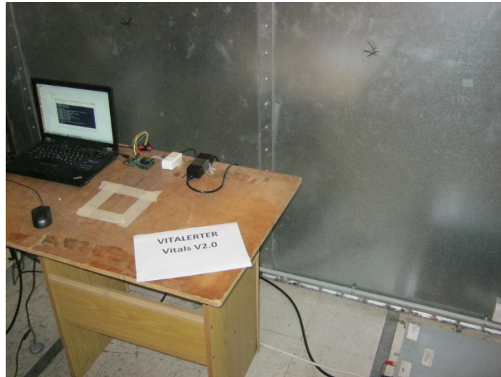
Figure 5. Conducted Emission from AC Mains Test
