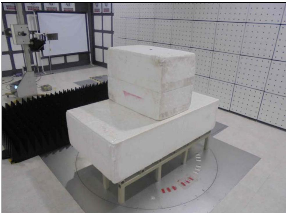
RADIATED EMISSION TEST (Mode B)
