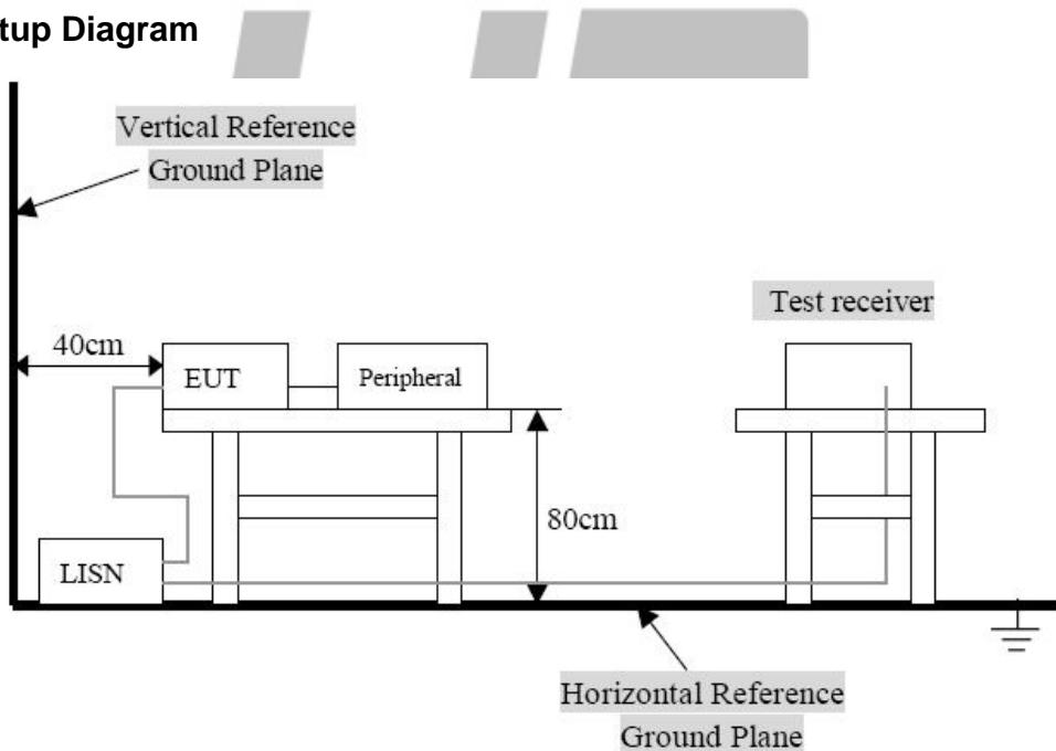
Remark: The EUT was connected to a 120VAC/ 60Hz power source.
