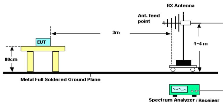
For radiated emission from above1GHz
