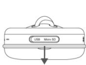
You can push the silicone strape towards the concave to take it out easily.
