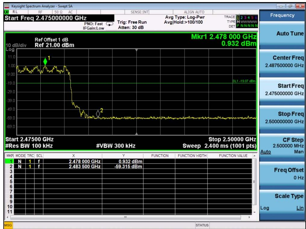
EDR mode(8DPSK): Band Edge-Left Side
