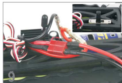
8 Be sure to first open the remote control power, and then open the model car power supply, switch on the power, the motor delivering a diz ~ diz ~ ~ sounds, it means the motor for standby state. open radio button, the motor will begin to run.
