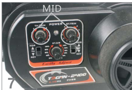
7 Adjust the throttle, steering vernier adjustment knob button to median (MID) direction. big/small rudder Angle knob button to 120%
