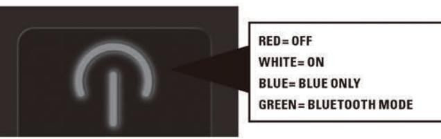
**Illuminated Touch Switch:** Switch changes color to indicate the different settings: off (red illumination), all lights on (white illumination), Blue lights only (blue illumination), Bluetooth mode (green illumination).
