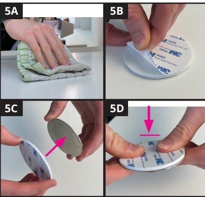
**EN** Choose a location to mount the camera. First clean and dry the surface, so it's free of any dust and debris. The sticker will only adhere to smooth, rigid surfaces. Peel off the foil on one end of the double-sided sticker, apply it to the metal disc and press it down evenly for 10 seconds.
