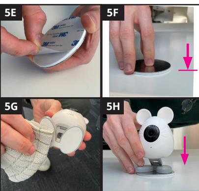
**EN** Peel off the foil on the other side of the sticker. To apply, press the sticker onto the surface for 10 seconds. **Ensure the anti-skid layer on the camera's feet is clean and free of dust.** Place the camera onto the metal disc with magnetic feet facing down.
