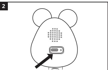
**EN** Insert the USB cable into the port at the back of the camera body.
