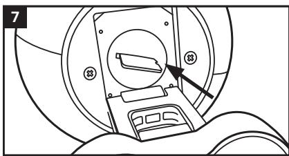
**EN** **RECOMMENDED:** Insert a micro SD-card (max. 128GB storage) in the slot at the bottom of the camera for data storage and automatic video recordings.
