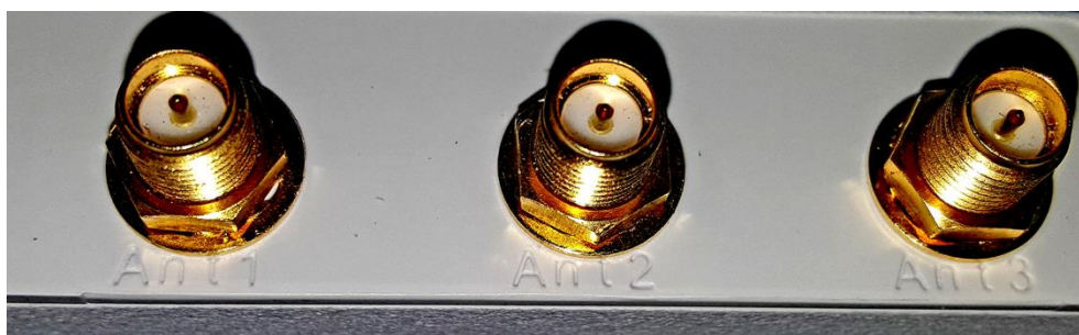
Figure 9: The three reverse-polarity SMA connectors for external antennas.
