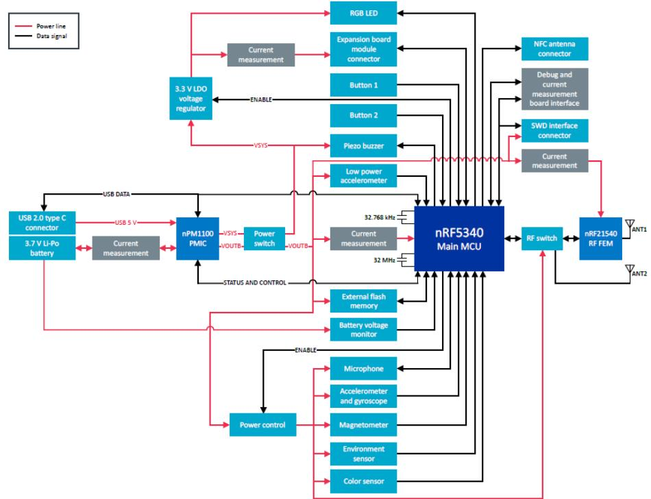
Figure 2: Nordic Thingy:53 hardware block diagram
