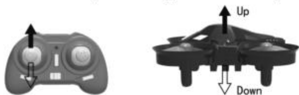
The left joystick controls up/down of four-axis aircraft
