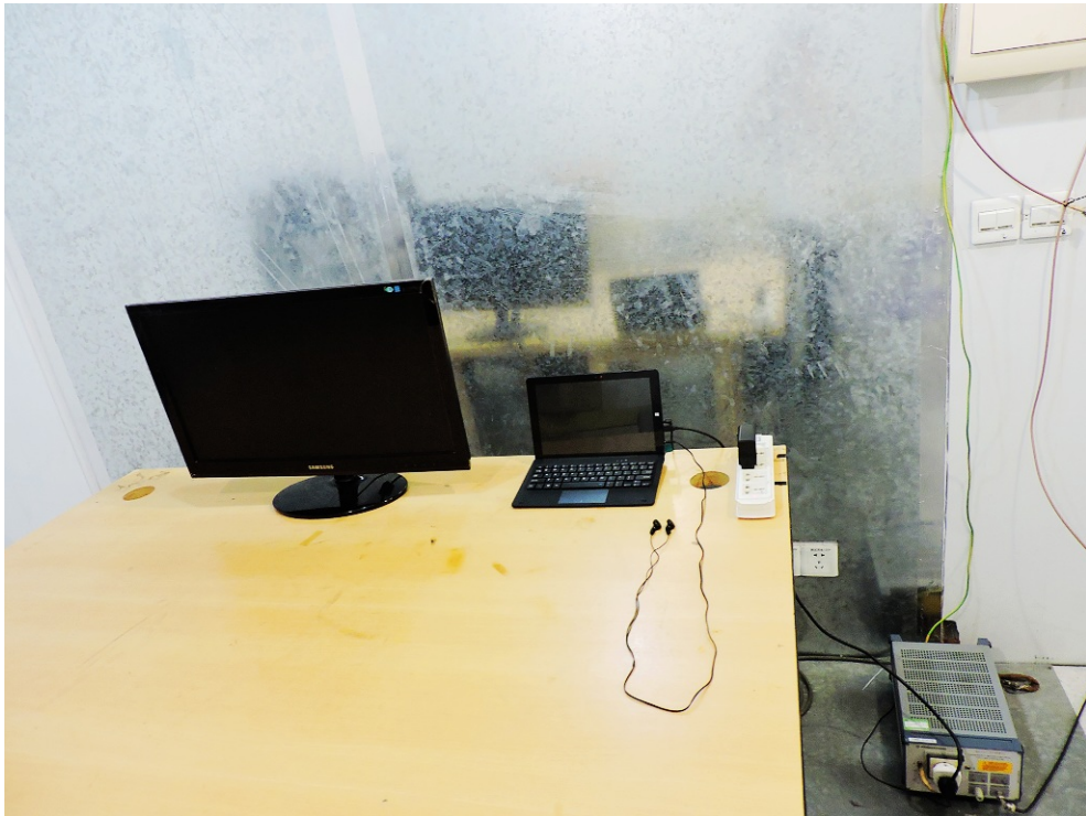
Conducted Emission Test Setup:
