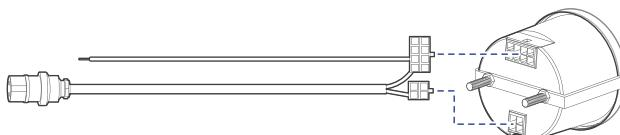
5. Connect the bare wire of the Battery Indicator Communication Cable to the negative end of the electric door lock on your golf cart. This ensures that the battery indicator will automatically turn on when the golf cart is powered on. You may refer to the golf cart user manual or consult the manufacturer for relevant information.
