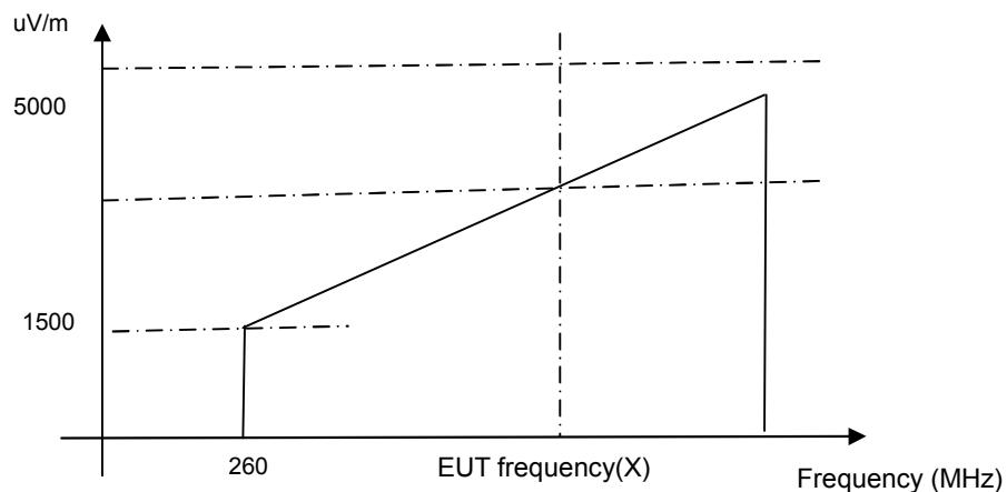
The Field Strength of Fundamental Emissions (Operating Frequency) is:
