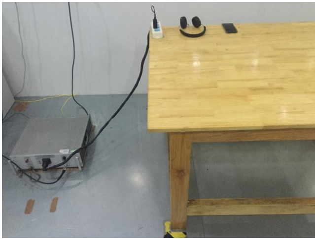
Conducted Emissions Test Setup Front View
