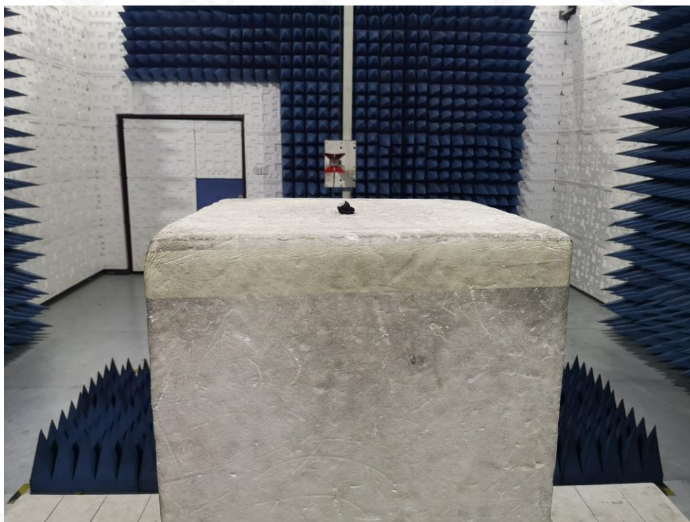
RADIATED EMISSION TEST SETUP ABOVE 1GHZ
