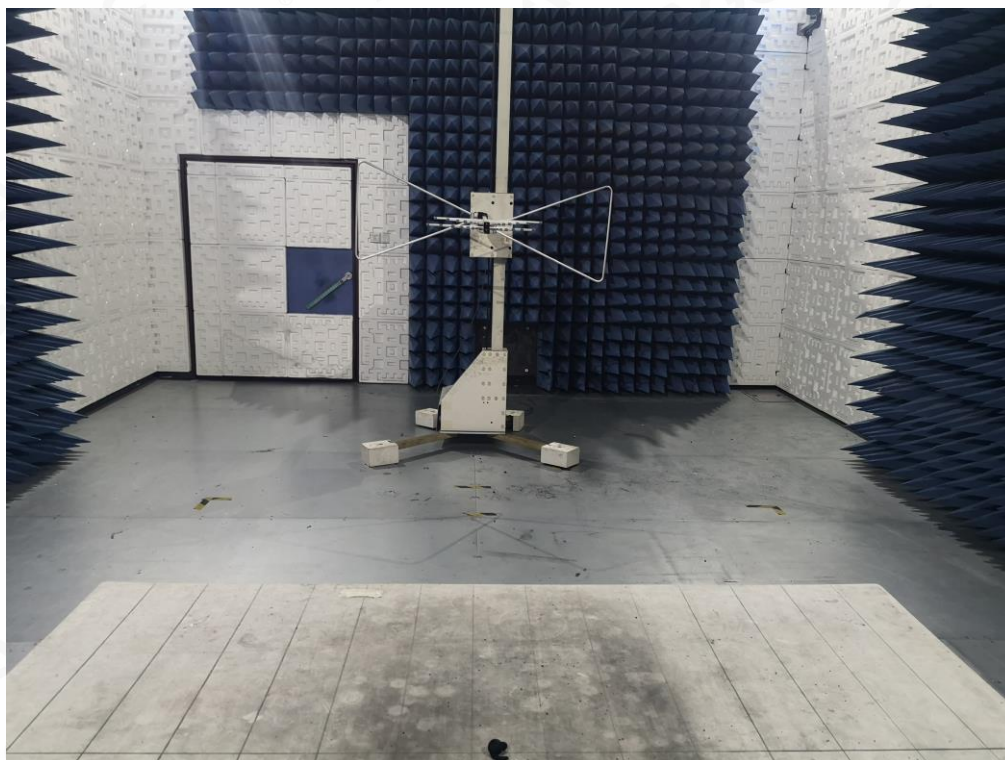
RADIATED EMISSION TEST SETUP ABOVE 1GHZ
